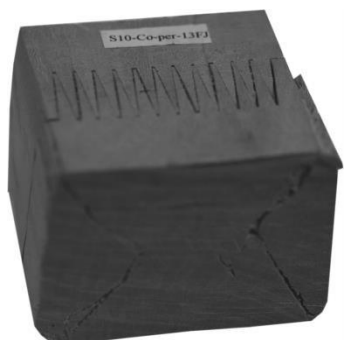
Figure-4b: Failure of the finger-jointed specimen under compression perpendicular to Grain.
