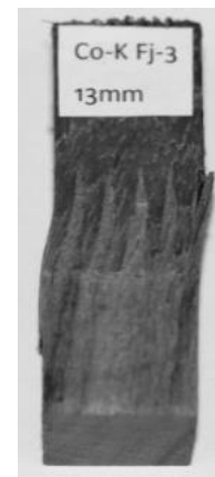
Figure-4a: Failure of the finger-jointed specimen under compression parallel to grain.
