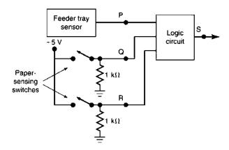
The presence of paper in the feeder tray is indicated by a HIGH at logic signal P. Each of the micro switches produces a logic signal (Q and R) that goes HIGH whenever paper is jammed over the switch to activate it.
