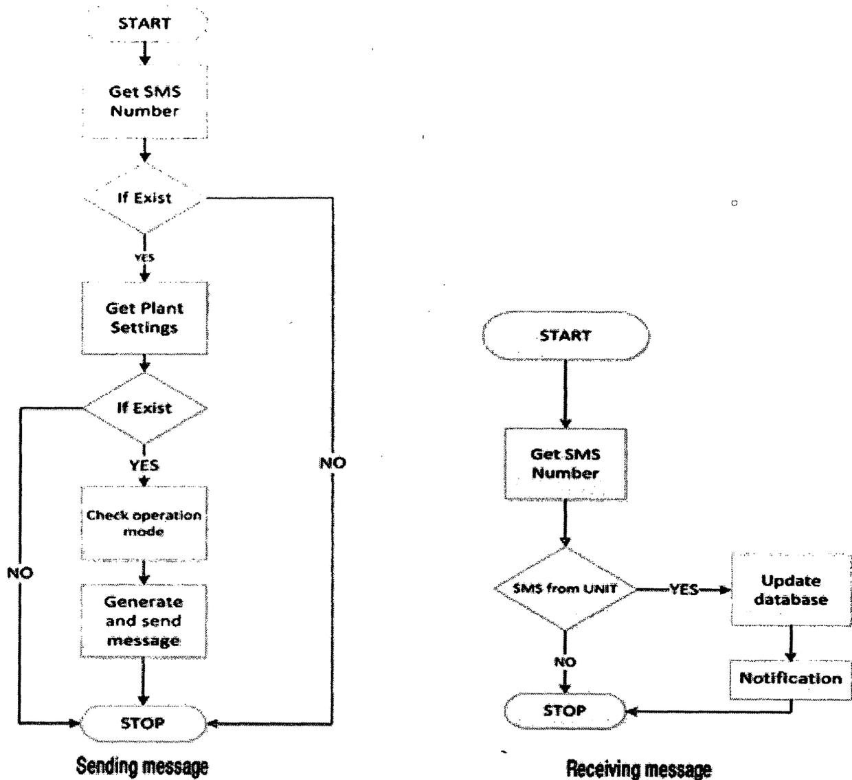
Figure 4. Algorithms for send and receive SMS through Android application
