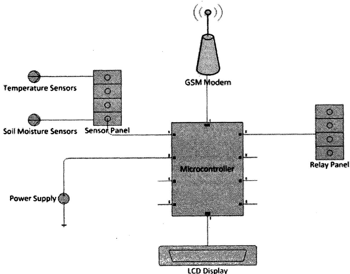
Figure 3. Connection diagram of overall controlling unit.
