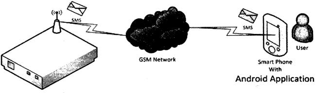
Overall Controlling Unit Figure 1. Basic setup of the system.
