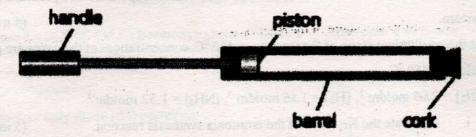
The air in the barrel is at a pressure of  $1.0 \times 10^5$  Pa, a temperature of 290 K and the volume is  $2.1 \times 10^{-5}$  m<sup>3</sup>. The volume of air in the barrel at the instant the cork is expelled is  $1.2 \times 10^{-5}$  m<sup>3</sup>.
