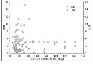
**Figure 7:** Variation of L/W and B/D ratios with Particle Reynolds Number  $(Re_p)$
