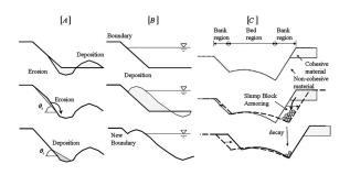
**Figure 2:** Bed deformation and concept of the armoring model[14]
