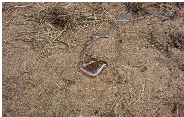
Figure 1: Water Applied on the surface flows through the slope without penetrating into the soil
