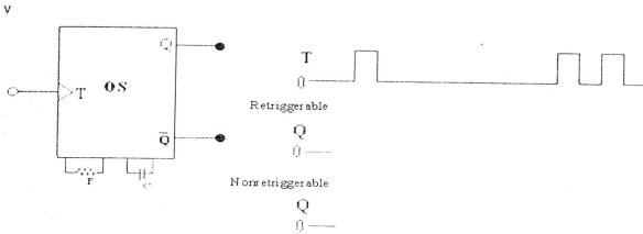
(Note: Quasi stable interval is 2 ms (> width of the clock pulse) for both cases)
