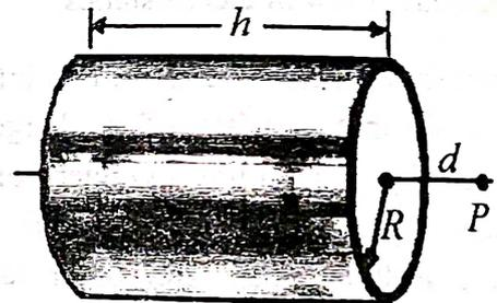
$$V = \left( \frac{k_e Q}{h} \right) \ln \left[ \frac{d + h + \sqrt{(d+h)^2 + R^2}}{d + \sqrt{d^2 + R^2}} \right]. \quad \left( \text{Note: } \int \frac{dx}{\sqrt{a^2 + x^2}} = \ln \left[ x + \sqrt{a^2 + x^2} \right] \right)$$
