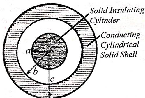
(i) Use Gauss's law to find an expression for the electric field  $\vec{E}_1$  at a distance  $r$ , ( $r < a$ ) from the axis of the cable.
