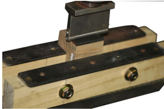
Fig. 2 Shearing tool used for the shear test
