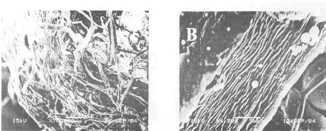
Figure 3. Scanning electron micrographs of used paper fibers, showing the micro morphology (A) Shows the porous structured arrangement of fibers (B) Shows micro morphology of binding surface of an individual Fiber.
