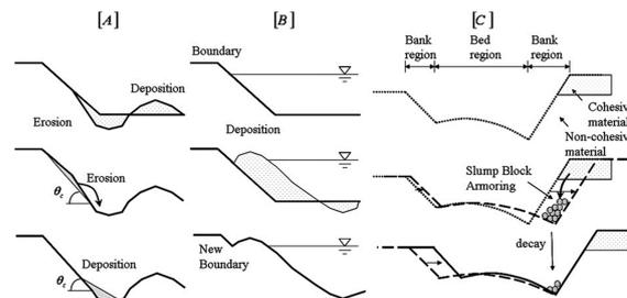
Figure 2: Bed deformation and concept of the armoring model[14]
