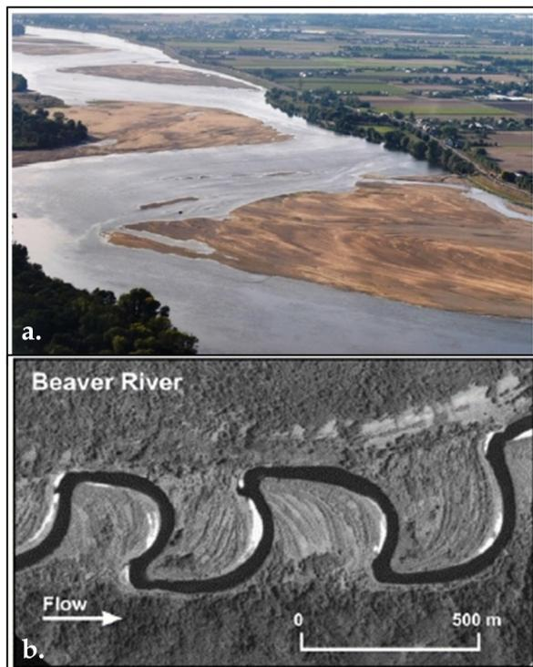
**Figure 1:** Alternate bars in the Loire River[2] b. meandering of Beaver River[5]
