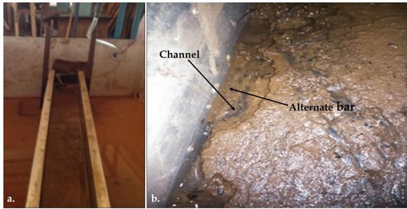
Figure 3: a. Experimental flume 1, b. Alternate bar and channel
