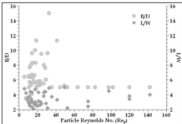
**Figure 7:** Variation of  $L/W$  and  $B/D$  ratios with Particle Reynolds Number ( $Re_p$ )
