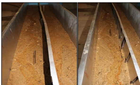
**Figure 5:** Occurrence of alternate bars in flume 2
