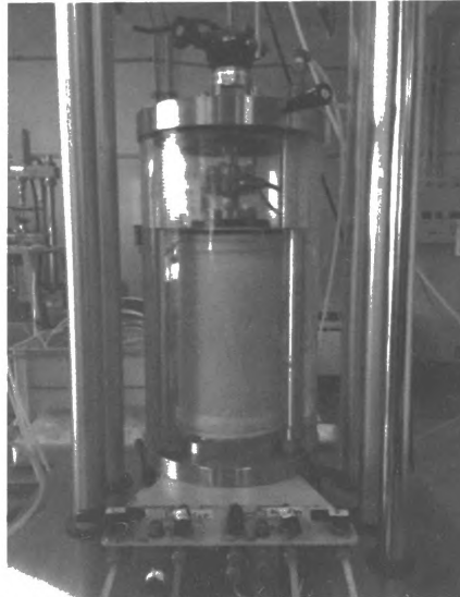
Figure 1 Experimental apparatus of triaxial compression test
