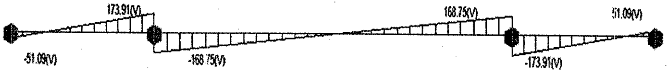
Fig. Q3 b) iii) Case 2: Alternative spans fully loaded maximum loading at the two edges
