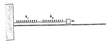
(a). Write down an expression for the effective force constant, Keff, for a single spring that could replace the two springs system. Hence show that the block exhibits a simple harmonic
