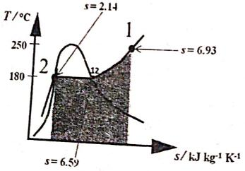
i. If the process is reversible, then estimate the heat transfer using the area in the T-s diagram. (Assume that the entropy changes linearly with temperature in the superheated
