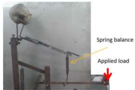
Figure 2: Experimental equipment for removing husk by broach
