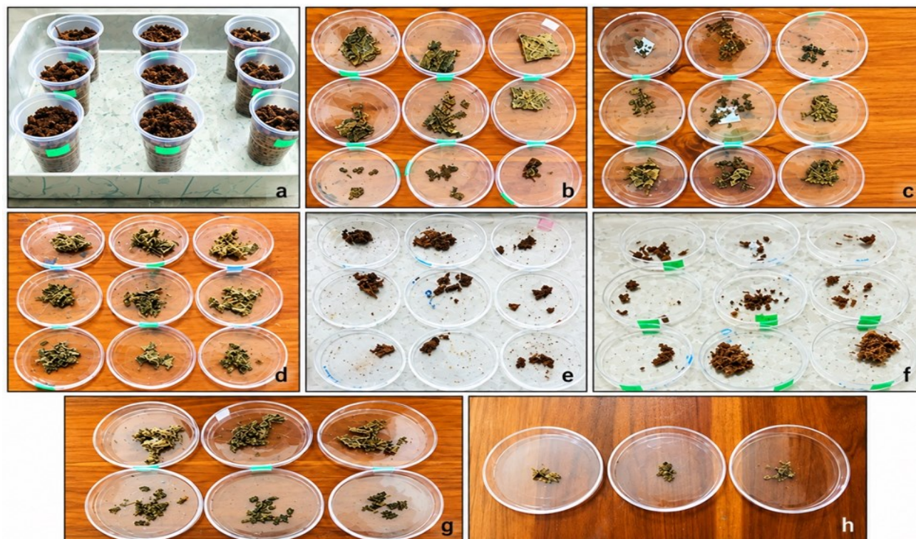
Figure 7: Visual progression of soil-burial degradation of T1–T3 biodegradable packaging sheets over 49 days: (a) 0 days, (b) 7 days, (c) 14 days, (d) 21 days, (e) 28 days, (f) 35 days, (g) 42 days, and (h) 49 days
