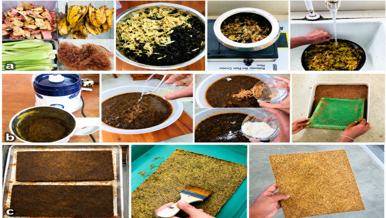
Figure 1: Sequential preparation of biodegradable fiber-based packaging sheets: (a) raw material preparation and pretreatment; (b) pulping, blending, and sheet formation; and (c) drying and application of cassava starch–PVA coating. T1:100 g, T2:200 g, and T3: 300 g corn husk content
